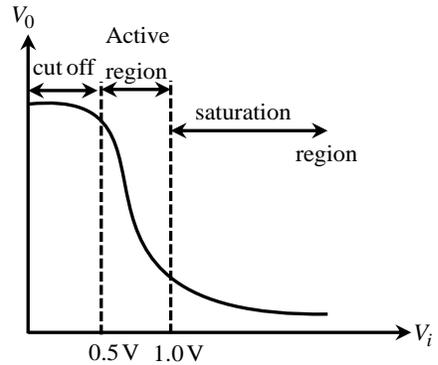
If we draw a graph of  $V_0$  against  $V_i$  we get a curve as shown in the figure. This graph is also called base biased transfer characteristics of a transistor. Now we will try to explain the action of transistor as a switch.
