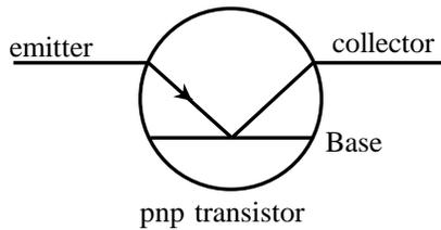
In the npn transistor, the current flows from base to the emitter. In the  $p$ - $n$ - $p$  transistor, the current flows from the emitter to the base. (1+1 marks)
